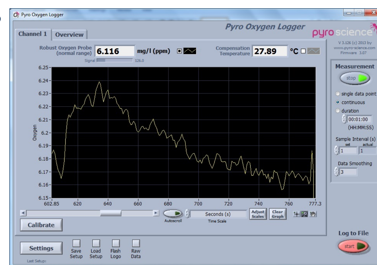
Figure 2. An oxygen readout from the data logger graphing a decrease in oxygen concentration in the swim tunnel over time.
