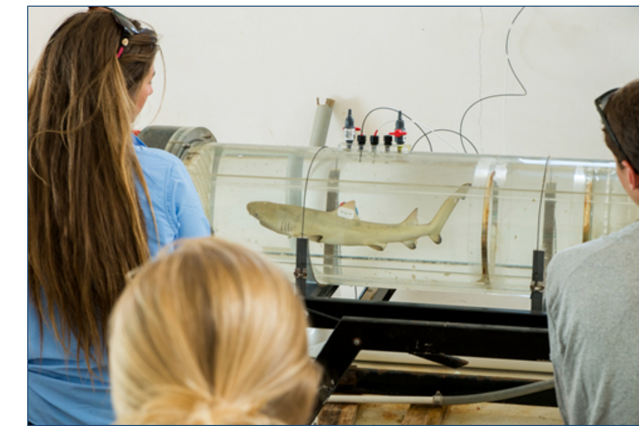
Figure 8. Juvenile lemon shark in a swim tunnel while oxygen consumption and acceleration were measured.
