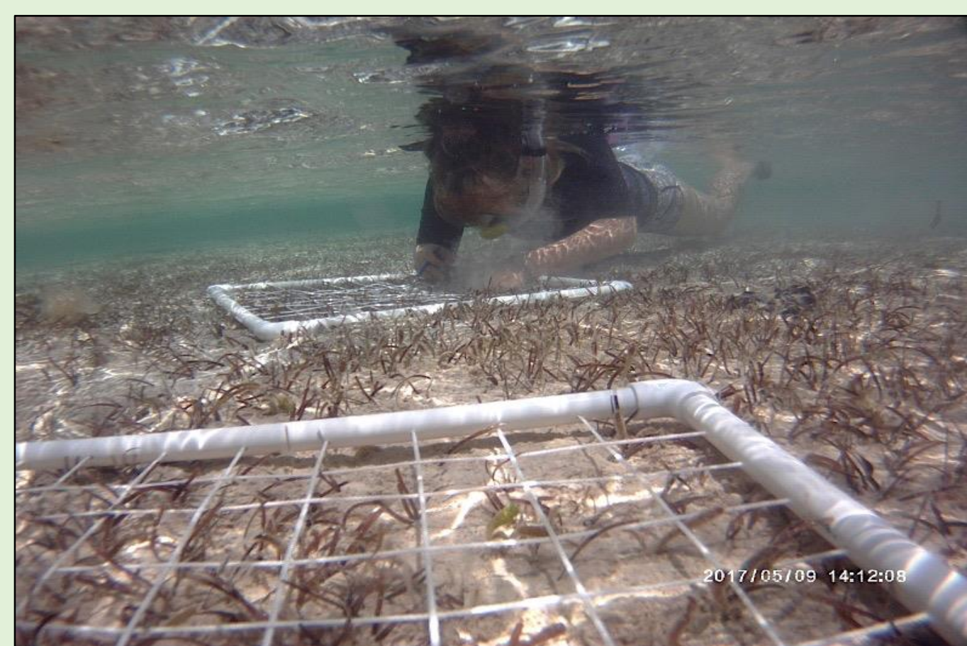
Figure 14: Research Advisor collects seagrass from a quadrat in Poison Creek that had been scarred two weeks prior to measure growth rate.
